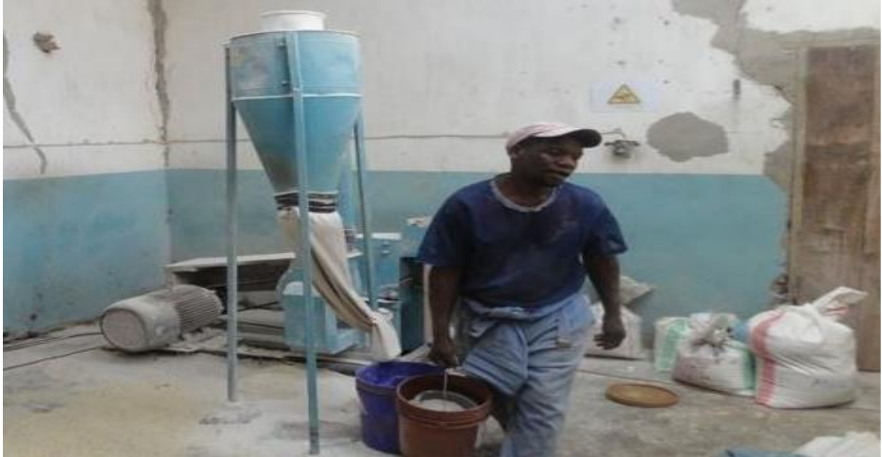
A typical hammer mill used for maize milling in rural areas of Tanzania (Photo credit: Joseph Mpagalile, FAO)
