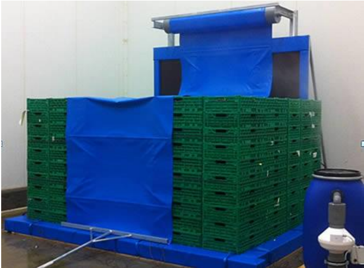
Larger scale pre-cooling unit, AB Speedbox Forced Air Cooler. Source: AB Coolservice (Belgium) www.abweb.be
