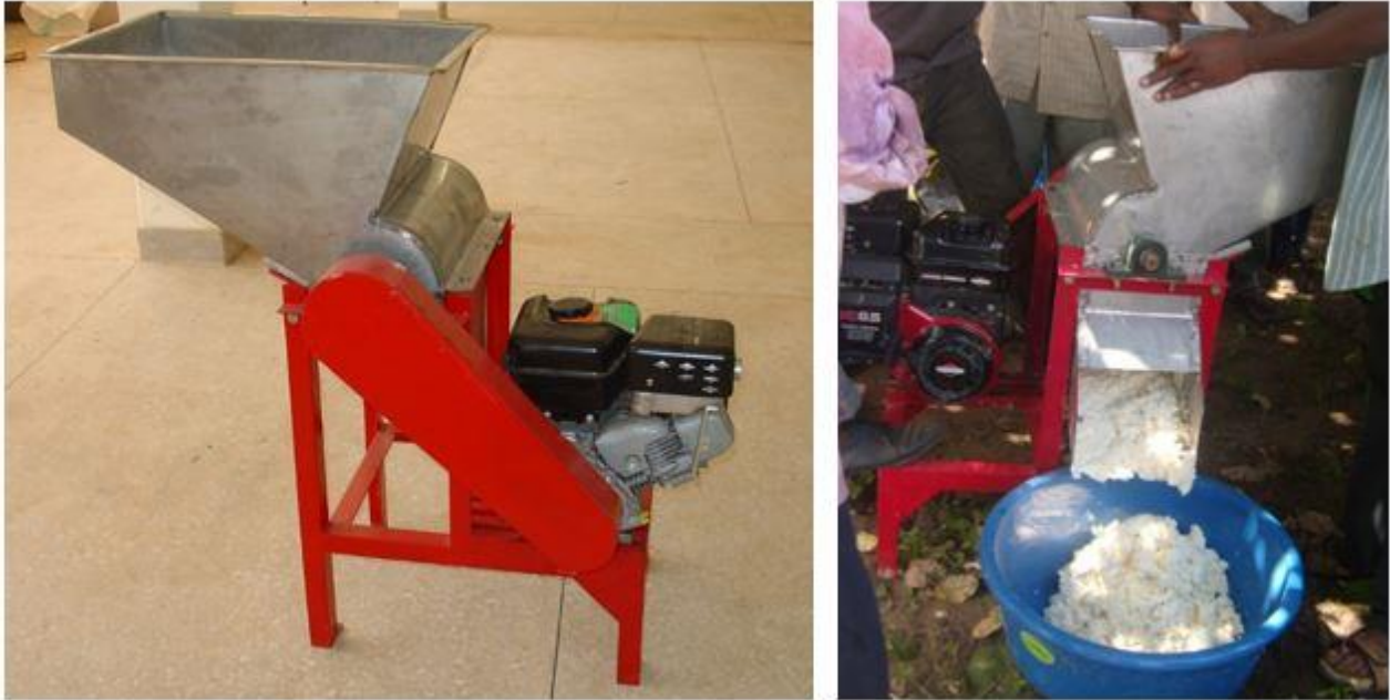
A motorized cassava grater manufactured by Intermech Engineering in operation in rural Tanzania (Source: Joseph Mpagalile, FAO)
