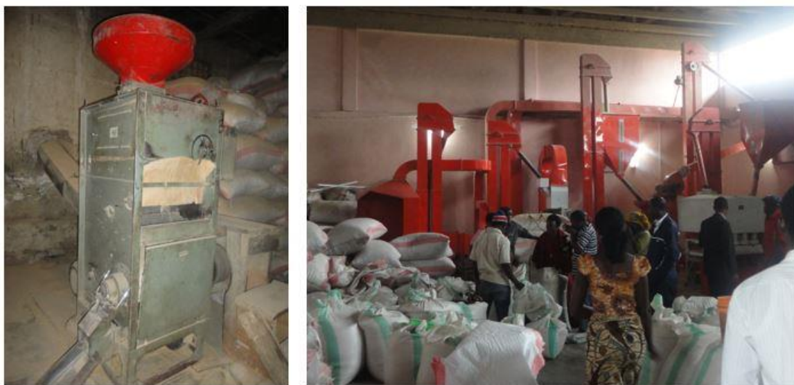
A small-scale rice dehusser (Left) and medium-scale rice milling machine capable of cleaning, dehulling and grading (Right) being used in Tanzania (Source: Joseph Mpagalile, FAO)
