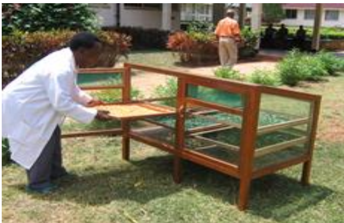
Solar drier in Tanzania (a direct model). Photo credits: Lisa Kitinoja
